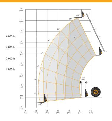
This load chart is for the rated capacity of the machine with 66" wide standard carriage and 48" pallet forks. Use only JCB approved attachments and check the relevant load chart for the machine model. If in doubt, consult your dealer. If the load rating of the machine differs to that of the attachment, the lower rating becomes the overall capacity.
