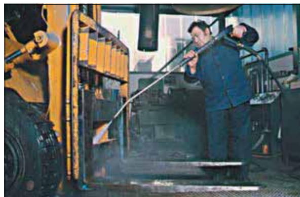
Hot water pressure washers are ideal for cleaning oil and greasy buildups from almost any surface.
