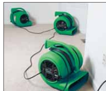
Dri-Eaz Sahara Pro X3 Turbodryers 3 units daisy-chained on a single 115V circuit
