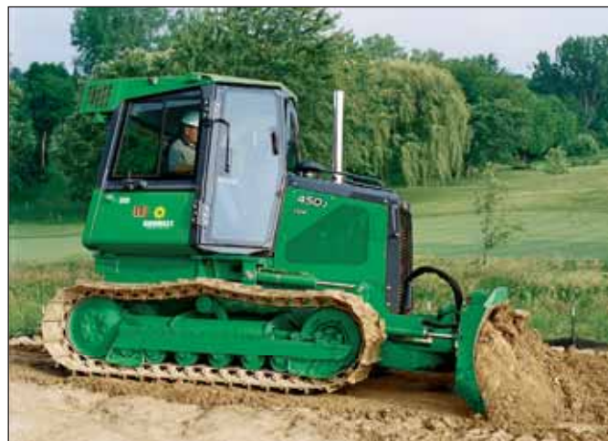
John Deere 450J 77 HP Crawler Dozer
