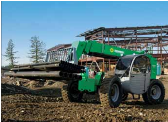
Genie GTH-844C 8,000 lb. Max Capacity, 44' Max Lift Height
