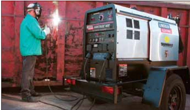
Lincoln Vantage 400 CC/CV 400A CC/CV trailer model
