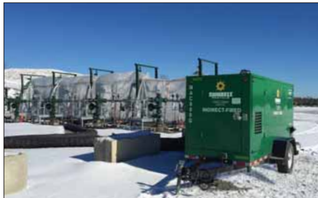
MAC 800G Indirect-Fired Heater Freeze protection for wellheads on an oil and gas site
