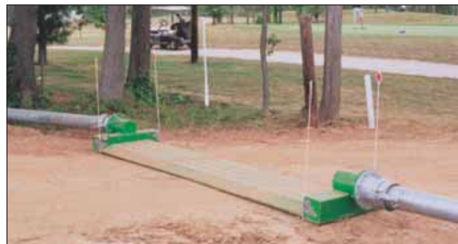
An 8" x 12' road ramp in operation on a golf course drought relief pump project
