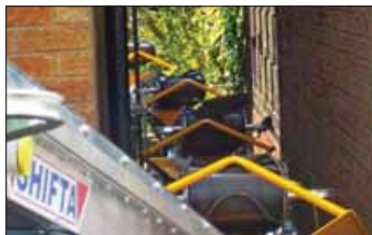
Sectional conveyors provide extra versatility for working in close quarters.
