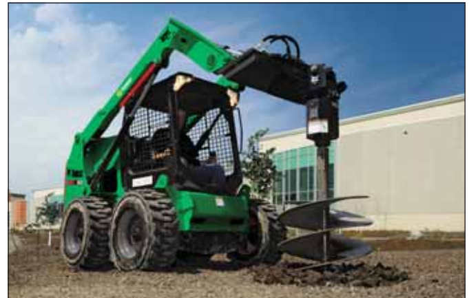
Bobcat S650 2,690 lb. Capacity, with Auger Attachment
