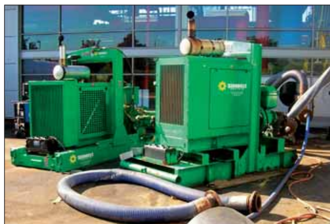
(2) Gorman-Rupp Diesel High Head Pumps
