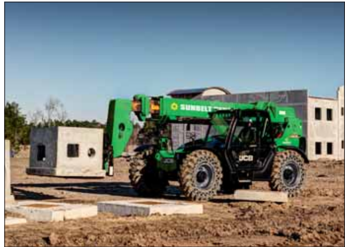
JCB 509-42 9,000 lb. Max Capacity, 42' Max Lift Height
