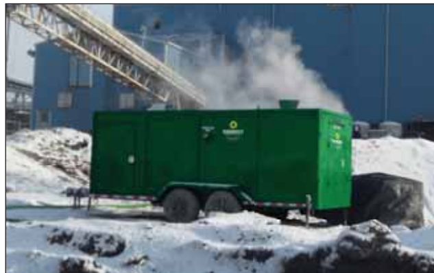
MAC Indirect-Fired Heater Temporary heat on an industrial site
