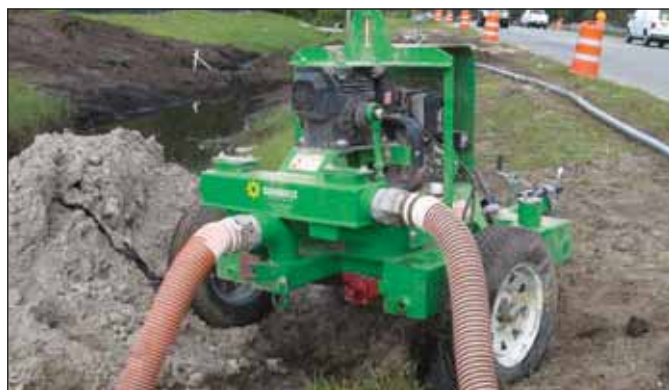
Myers-Seth DD-4/HA/T 4" Diesel Double Diaphragm Pump
