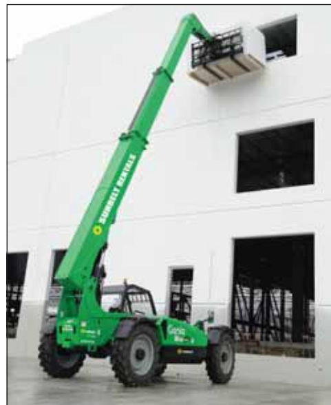
Genie GTH-636 6,000 lb. Max Capacity, 36' Max Lift Height
