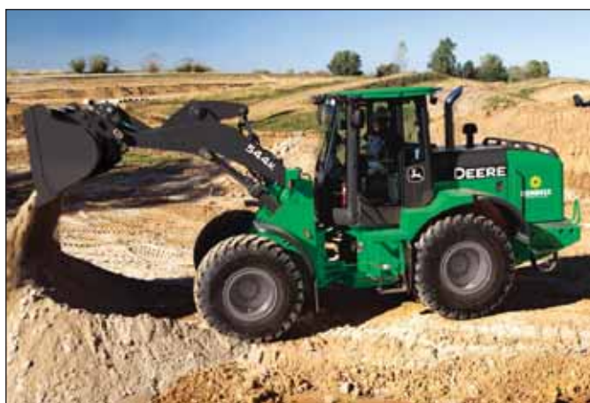
John Deere 544K 3 cu. yd. Wheel Loader
