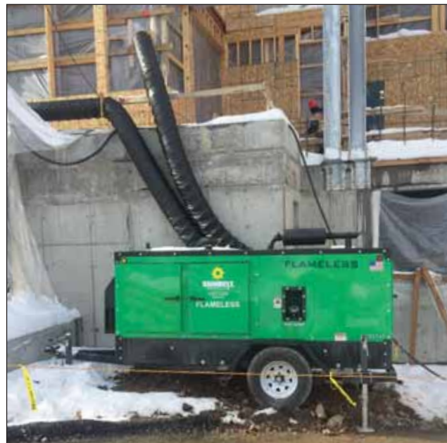
MAC 750F Flameless Heater Flameless heat for a commercial construction site
