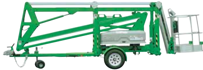
Boom folds down onto trailer for easy highway towing.
