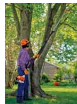
Stihl HT102 Pole Pruner Features a telescopic shaft
