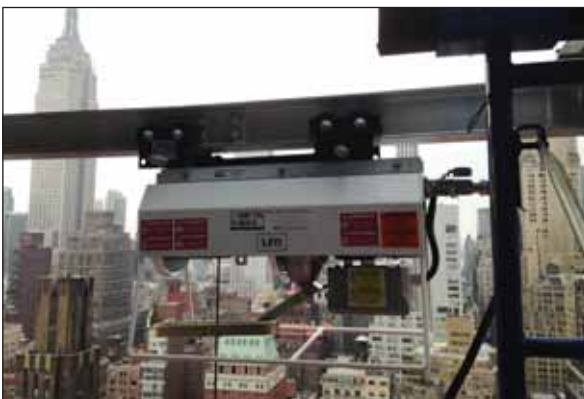
VFD Models provide a smoother start and stop which are ideal for hoisting materials, such as glass panels
