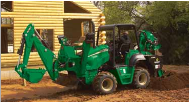
Ditch Witch RT75 w/BH 74 HP Ride-on Trencher
