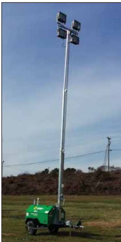
Terex RL4 4,000 watt Towable Light Tower Horizontal Mast Style
