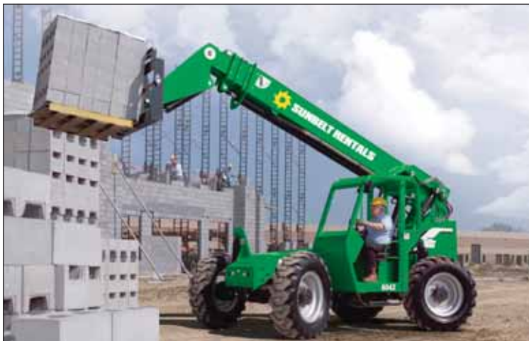
SkyTrak 6042 6,000 lb. Max Capacity, 42' Max Lift Height
