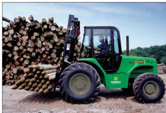
JCB 940 8,000 lb. 4WD Straight Mast RT Forklift
