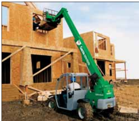
Genie GTH-5519 5,500 lb. Max Capacity, 19' Max Lift Height
