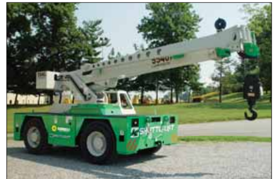
Shuttlelift 5540 15-ton Carry Deck Crane
