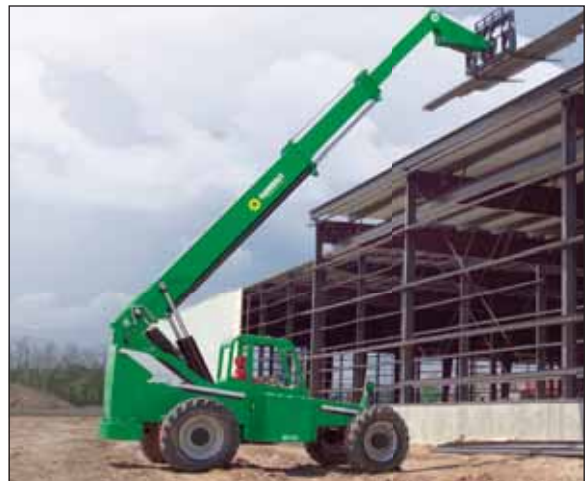
SkyTrak 8042 8,000 lb. Max Capacity, 42' Max Lift Height
