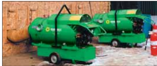
(2 Units) ICE OHV 350 320,000 BTU Oil Indirect-Fired Shown heating a temporary construction building
