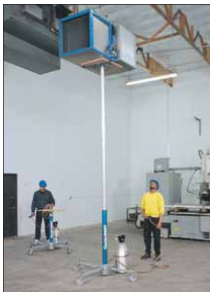
Genie GH5.6 18' Telescopic Lift Powered by CO 2 or compressed air
