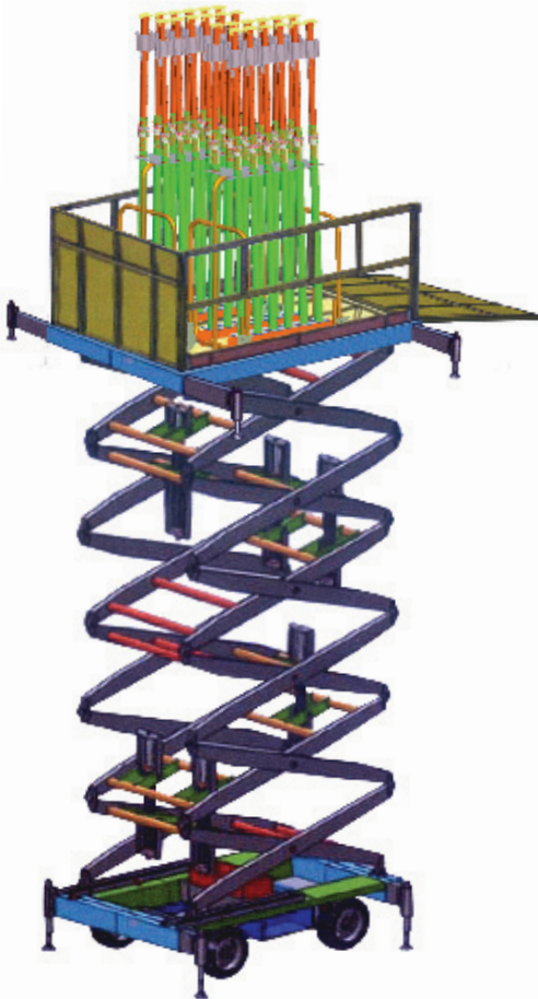
The TABLA Lifter self-propelled material lifter in extended position.
